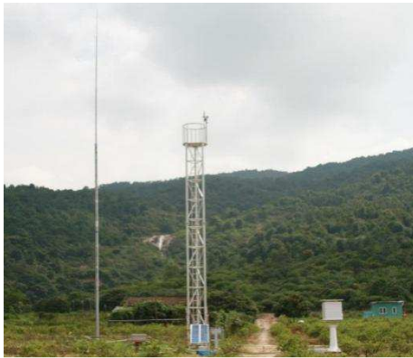
Fig. 8 Lightning protection experiment for AWS
