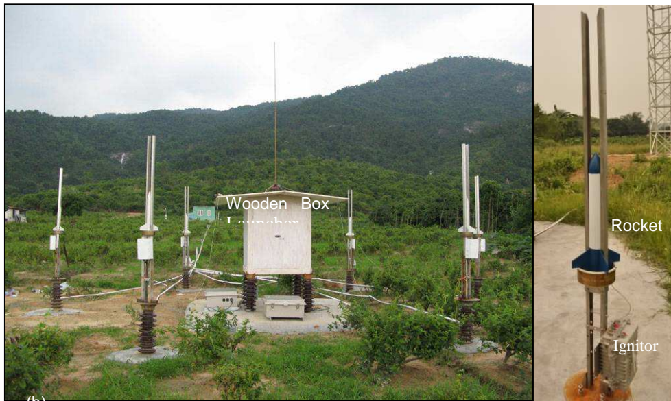
Fig.2 The field experiment site for triggered-lightning in Conghua. (b) Rocket launcher
